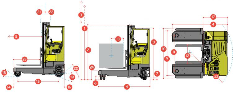
This compact truck features two rear wheel drive with rubber tyres and dynamic  $360^{\circ}$  4 wheel steering rotation, contributing to faster procedures for manufacturing, distribution and logistics operations.
