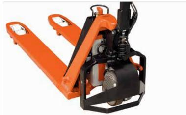
The LHT100's motor and battery are compact enough for it to be as manoeuvrable as a standard BT Lifter
