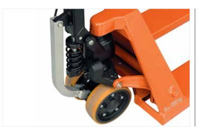
The BT Pro Lifter's steering arm provides leverage to the wheels to help get the truck moving
