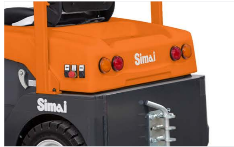
Inching buttons to slowly back up to connect to load carrier.
