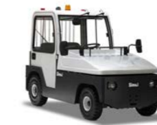
The TE250R model is suited for heavy-duty work up to 25 tonnes. With the bonnet at the front, the rear visibility is excellent.
