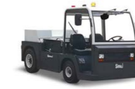
With 50-tonnes towing capacity, the TE500RR range is designed to tow heavy parts in the automotive, steel or any other heavy-duty industry.
