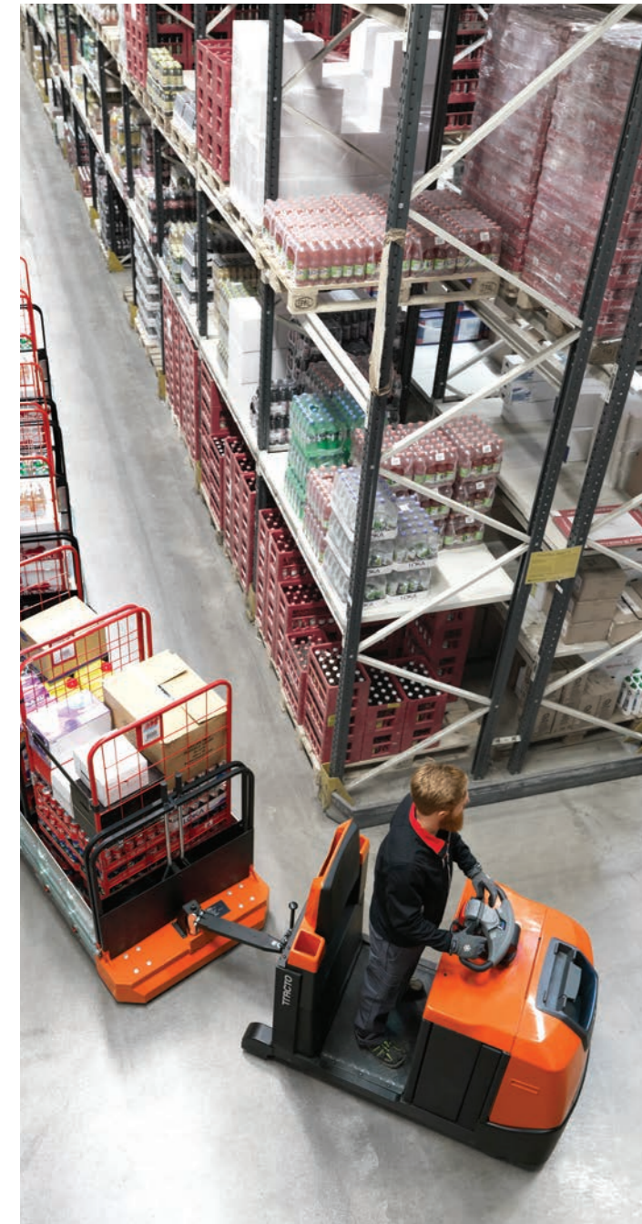
Low step-in and optional vibration-damped floor.
