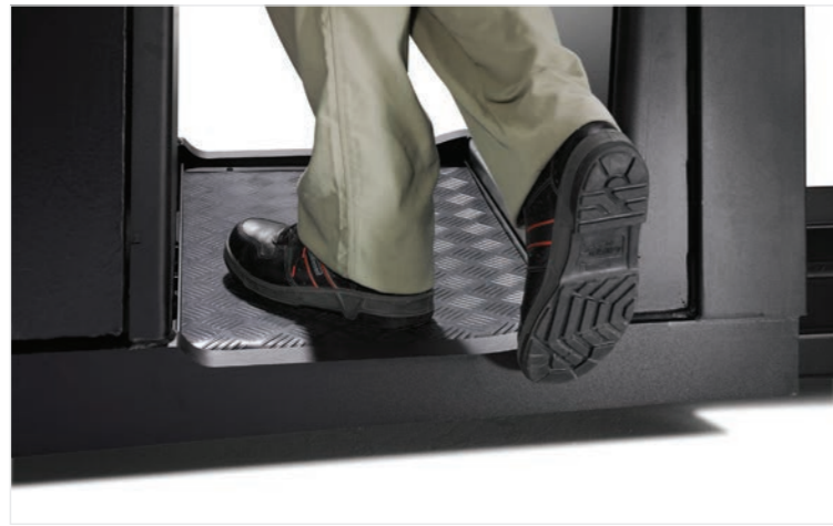
Low step-in and optional vibration-damped floor.
